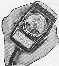
Baffle drops at touch of button to read incident light in foot-candles.
